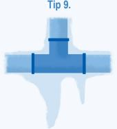
Prevent your water pipes from freezing this winter, by placing an infrared bulb and frost thermostat in your attic that's set to switch on at -3°C and turn off again when the temperature rises. This handy trick will help prevent your water pipes from freezing.
